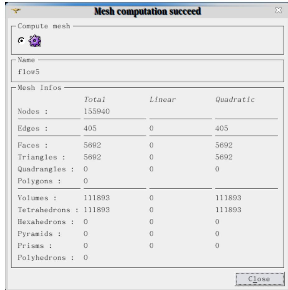
The screenshot shows a dialog box titled "Mesh computation succeed" with a close button (X) in the top right corner. The dialog contains a "Compute mesh" section with a gear icon, a "Name" field containing "flow5", and a "Mesh Infos" section with a table of mesh statistics. The table has columns for "Total", "Linear", and "Quadratic" mesh types. The statistics are as follows:
