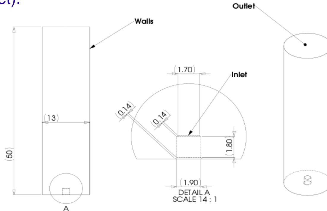
This is exported from SolidWorks in STEP file format and assigned groups in Salomé geometry module, before it is meshed in the meshing module using the following parameters
